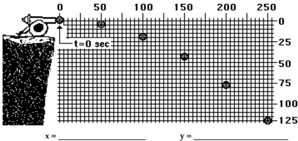
6. A ball is launched horizontally from the top of a cliff with an initial velocity of 20 m/s. The trajectory of the ball is shown below. Express your understanding by filling in the blanks.
